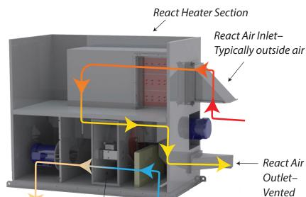
Rotor Supply Inlet – to be dried Supply Air Outlet-Dehumidified, dry air
